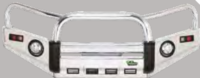
PREMIUM ALLOY 75mm inner and 50mm outer loop bars
